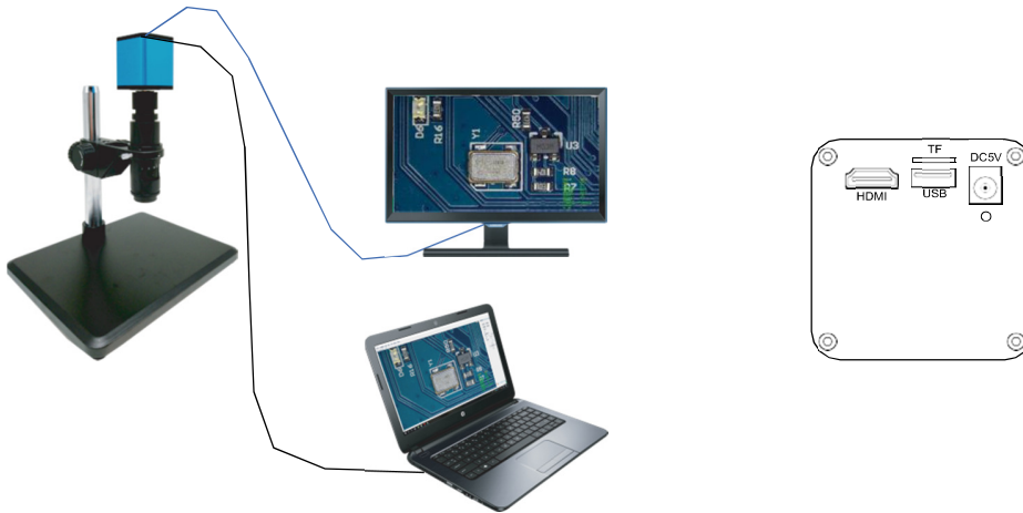
Picture 3: EA304 HDMI+USB Dual Output
